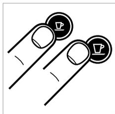
1. To enter the emptying mode, press both the Espresso and Lungo button to turn the machine off.
