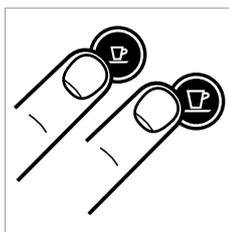
5. To enter the descaling mode, while the machine is turned on, press both the Espresso and Lungo buttons for 3 seconds.
