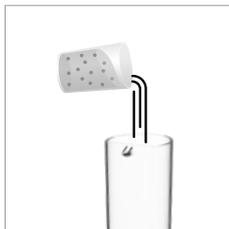
7. Refill the water tank with the used descaling solution collected in the container and repeat step 4 and 6.
