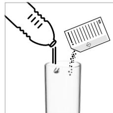
3. Fill the water tank with 0.5 L of fresh potable water and add 1 Nespresso descaling liquid sachet.
