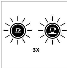
2. LEDs will blink fast 3 times to confirm machine has been reset to factory settings.
