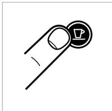
1. With the machine OFF, press and hold down the Lungo button for 5 seconds.
