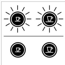
3. LEDs will then continue to blink normally, as heating up, until ready.
