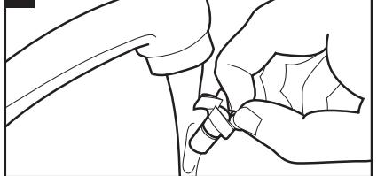
**EN** Rinse each part with water, removing any hairs or debris from the impeller and pump housing, before carefully reassembling.
