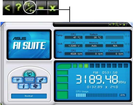
The image shows the ASUS AI Suite interface with a callout box highlighting the temperature unit icon (a circle with 'C' and 'F') in the top right corner of the main window. The monitoring window displays the same data as in the previous image, but the temperature units are now in Fahrenheit:
